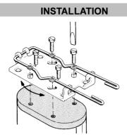
Depending on the structure of the mast, fix the base plate on the mast top, using suitable screws. Rotate the base plate over the oblong holes so that its central axis is parallel to the longitudinal ship axis, or to port or starboard. Inclinations of the mast top can be compensated with the sensor footplate.
