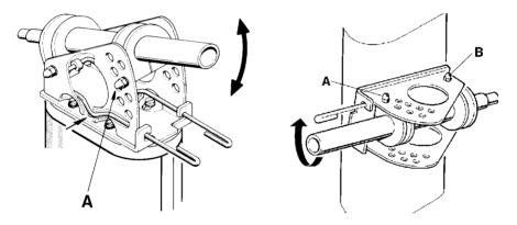
Install the sensor on the base plate. Sensor inclinations can be compensated by changing pin and nut (A). In the case of lateral mast mounting loosen the nuts (A) and (B) and turn the sensor so that it is vertical to the midship axis.
