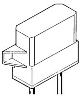
Install the cable socket below deck at the foot of the mast as shown. The socket must be protected against water damage. Make all screw connections with care. The cables shall leave the socket downward.
