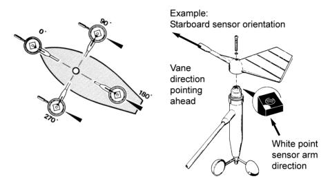
When mounting the base plate, the sensor mounting direction should be pointing ahead  $(0^{\circ})$  if possible. If this is not possible, other mounting directions can be used  $(90^{\circ}, 180^{\circ}, 270^{\circ})$ .
