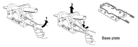
Loosen the spring clip by pushing it down and inward (1), (2), then remove the wind sensor (3).
