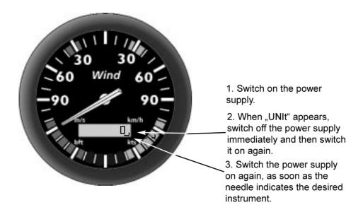
On power up, the instrument shows the text "UNIt" for 5 seconds. Switch off the power supply before this time elapses and switch it on again.
